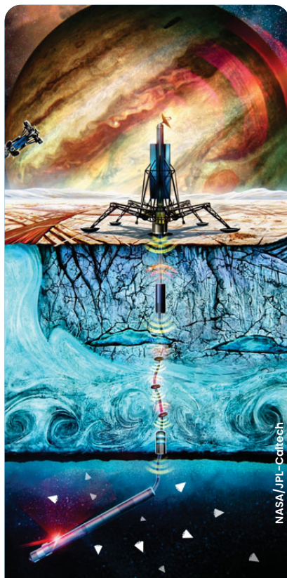
This illustration shows how a landing craft could send a heated probe through the ice to release the SWIM robots into the water
